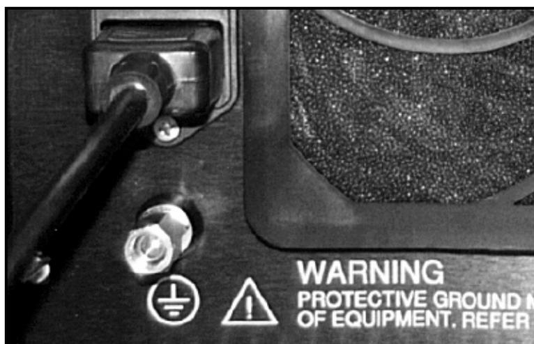
Figure 4. MULTI-TRACER Ground Connector.
